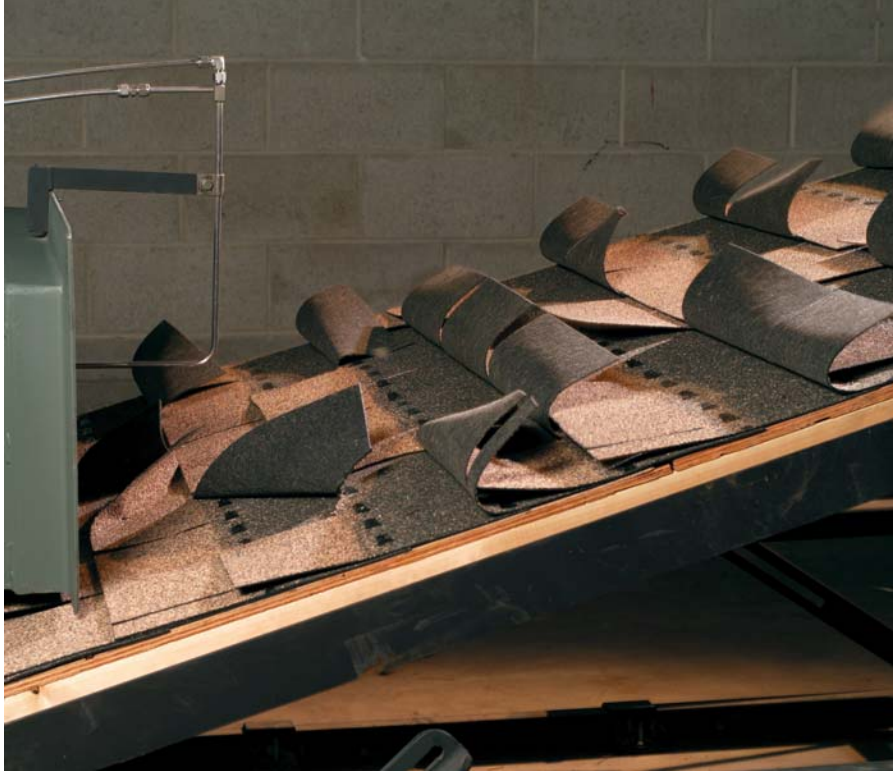
Shingles are tested under high wind conditions at the testing facility.
